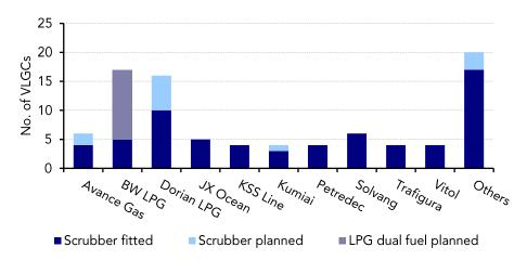
In terms of type of scrubbers, open loop scrubbers appear to be more popular. Out of 66 VLGCs that have scrubber fitted onboard the vessel, whether yard-fitted or retrofitted, 80% have open loop scrubbers. The rest are hybrid types. Out of the 12 VLGCs that are currently planning to install scrubbers, 64% will have open loop type scrubbers.
